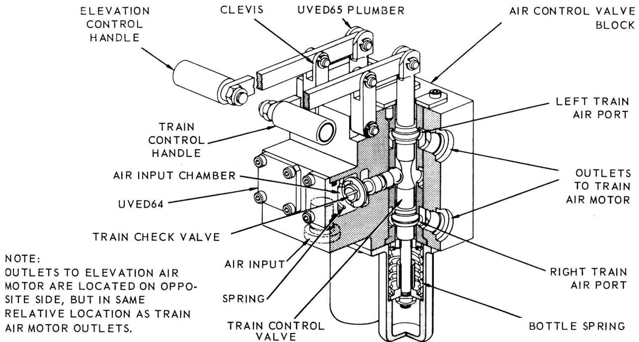
Figure 7-6.—Schematic of air motor drive.
